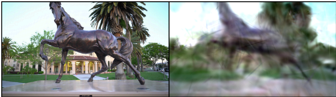
Figure 9: Comparison of the pre-optimized truth image (left) and the optimized Gaussian model using the optimizer's renderer(right) from a horse image set.
